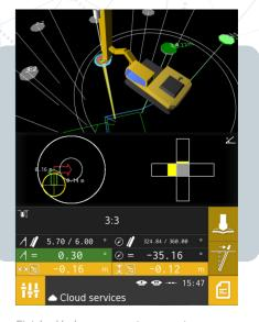
Finished holes are easy to separate from the system's screen from the green color.
