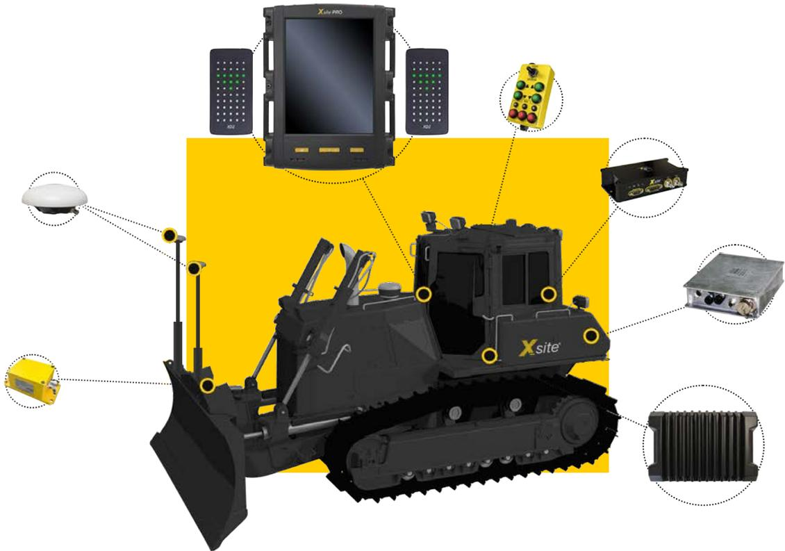
Components: Blade sensor, GNSS masts, GNSS antennas, Display unit (8,4"), 2 x LED-Display, Blade control unit, GNSS receiver, Hydraulics controller, Control unit (MC)
