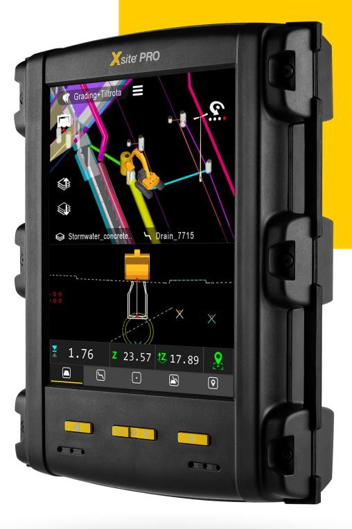
With Xsite PRO 3D the operator can select and view the models as one user-friendly entity, with clear naming.
