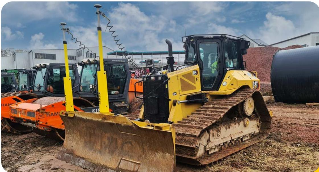
Xsite® PRO enables you to harness the efficiency of 3D machine control even in every project. The operator can easily create e.g. a sloped plane model using the built-in model tools. This speeds up the construction process remarkably - No need for manual grade checking or waiting for a surveyor.
