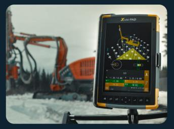
The accuracy of the Xsite DRILL system is up to +/- 30 mm. This is based on satellite positioning (GNSS) and a correction signal either from a local RTK base station or from a mobile VRS network.
