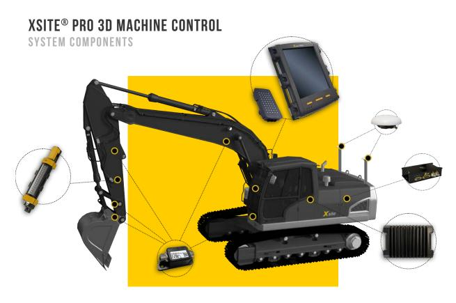
Components: Laser receiver (optional), Tilt sensor (optional), Bucket sensor, Boom sensor, Arm Sensor, Frame sensor, Display unit (8,4"), LED-Display (optional), GNSS masts, GNSS antennas, GNSS receiver, Control unit
